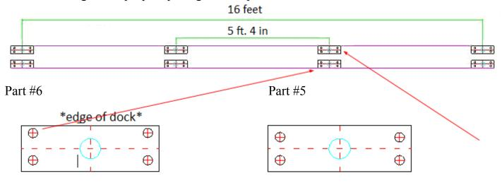
Base-Plate with holes closest to edge to be mounted on dock edge closest to water.
