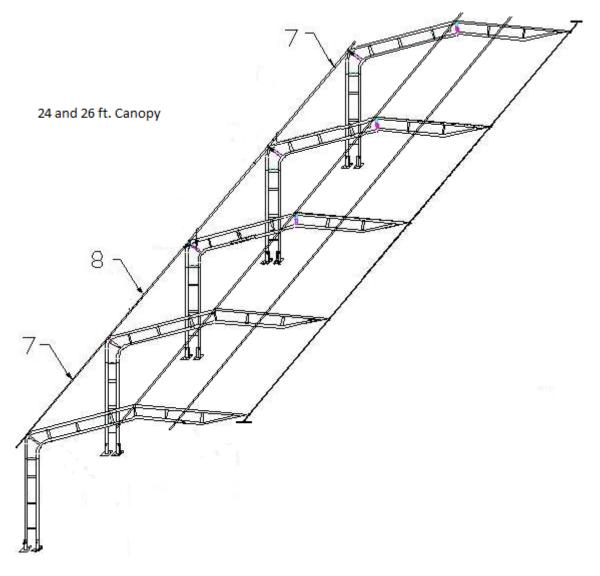
WARNING: DOCK MUST BE ANCHORED SERCURELY AND WEIGHTED SUFFICIENTLY ENOUGH TO WITHSTAND THE FORCES OF WINDS AGAINST THE CANOPY **<u>STEP 1</u>**: Fix the base plates #5 and #6 on the dock.
