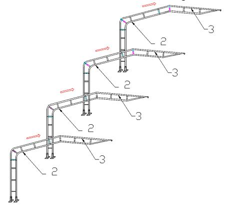
**STEP 4:** Fix clamp #9 and support tube #4 with the bolts #10. Bolts on support tubes must remain loose until the purlins are installed. Put the purlins (rods) #7 and #8 into support tube #4 and the clamps and tighten bolts. Install center perlins into clamps as well.
